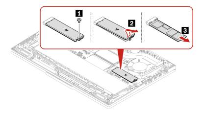
Step 2. Install the solid-state drive and its bracket in reverse order.
