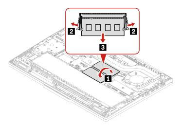
Step 2. Install the memory module as shown below.
