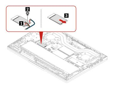
**Note:** A Mylar film might cover the wireless WAN card. To access the wireless WAN card, peel off the film first.
