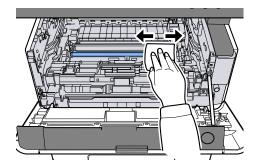
7 Slide the charger cleaner knob on the upper side of the drum unit left and right 2 or 3 times.
