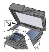
2 Align it flush against the original size indicator plates with the back left corner as the reference point.
