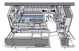
7 Slide the upper charger cleaner knob of the Drum unit to the left and right two or three times.
