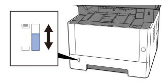
Remove the paper from the cassette once if there is no improvement, turn it over and reload it, or change the loading direction by rotating the paper 180 degrees.
