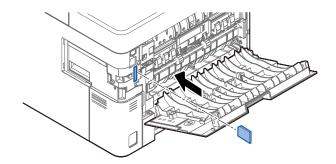
⚠ Attach the removed cover to the main unit.
