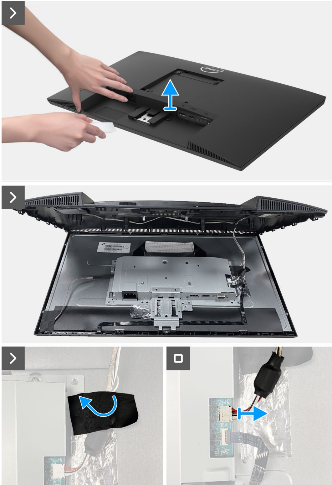
Figure 14. Removing the back cover
