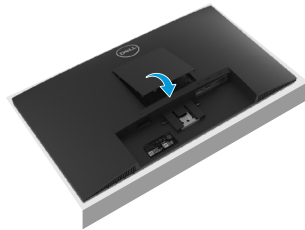
Figure 17. Assemble the VESA cover
