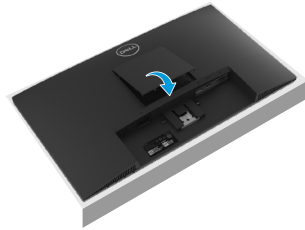
Figure 14. Assemble the VESA cover
