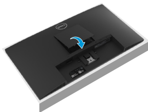
Figure 14. Installer le couvercle VESA
