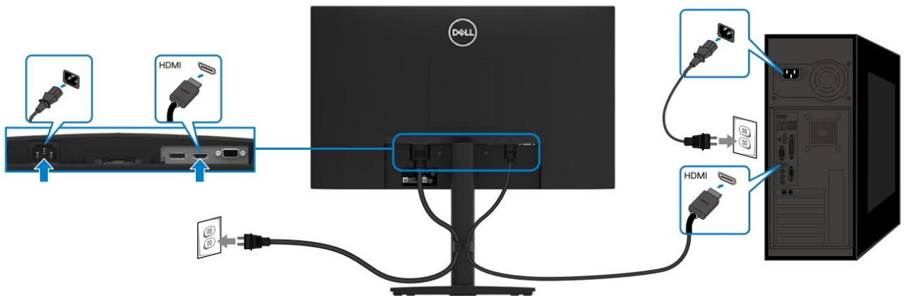
Figure 8. Connecting HDMI cable
