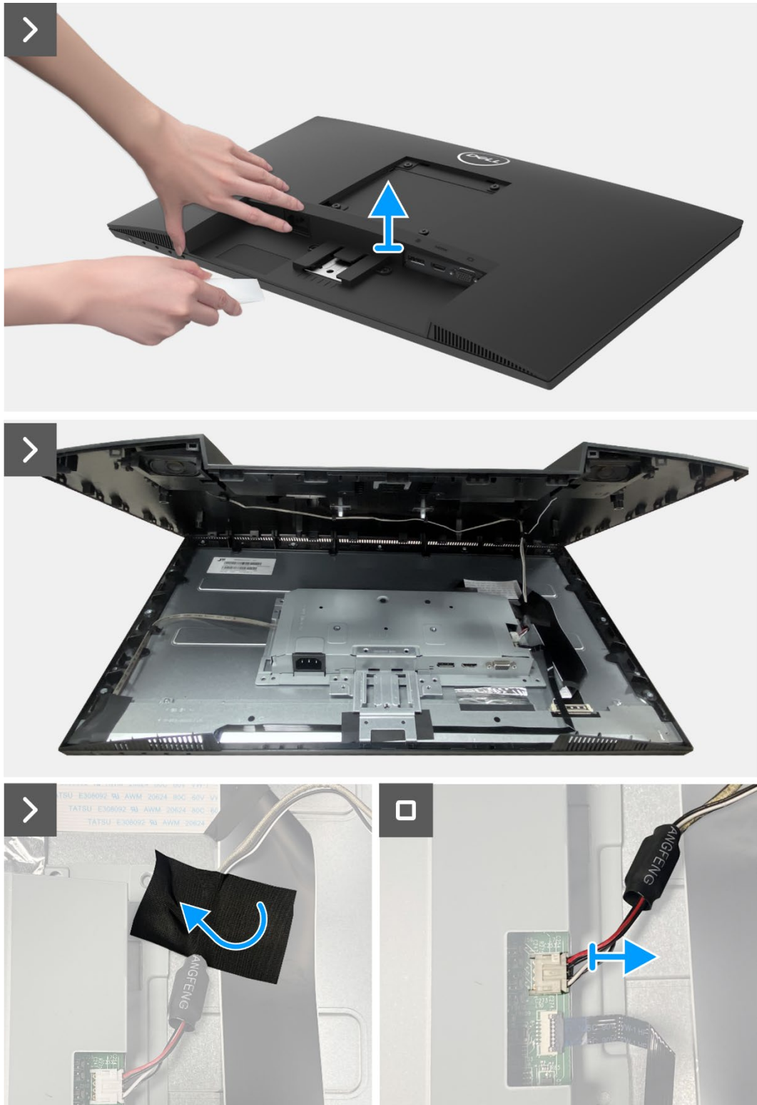
Figure 14. Removing the back cover
