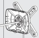
Remove the Shell Fixing Covers. Feed the Flat Cable into the assembly & locate the Tablet in the chosen orientation.
