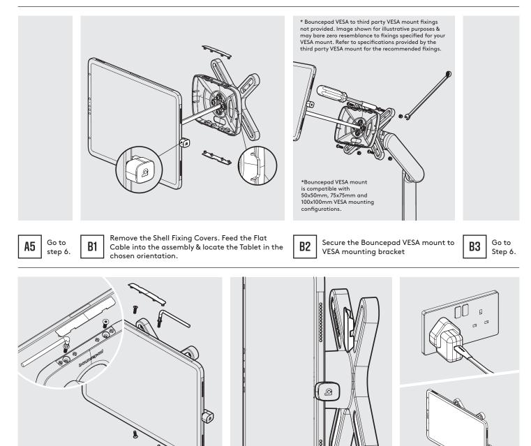
Secure the Tablet to the Shell & attach the Shell Fixing Covers as shown.
