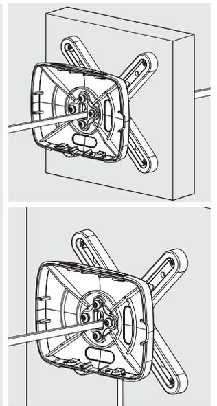
**A3** Remove the Shell Fixing Covers. Feed the Flat Cable into the assembly & locate the Tablet in the chosen orientation.
