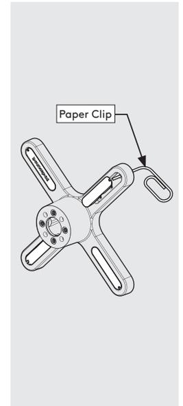
**1** Remove the Mounting Plate adhesive backing. Attach level & centrally to the Tablet back as shown.
