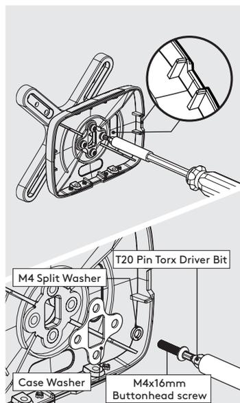
**5** Locate & attach the Shell to the Wallmount in the correct orientation.
