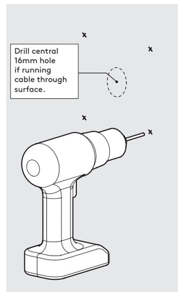
**A2** Drill the fixing holes into your surface.
