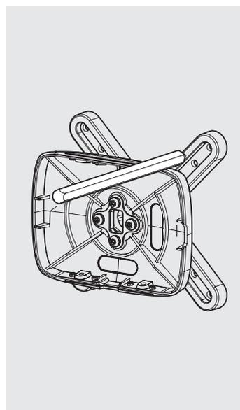
**A1** Position & mark where the VESA is to be located. Ensure the VESA is level.
