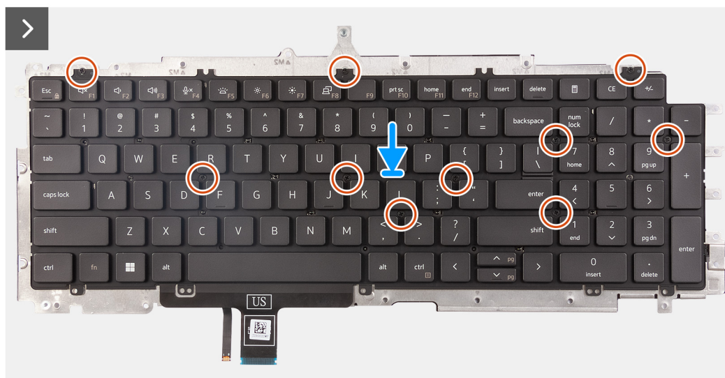
Figure 67. Installation du clavier
