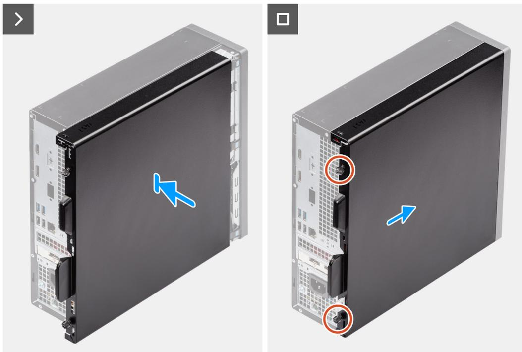
**Figura4. Instalar a tampa lateral**
