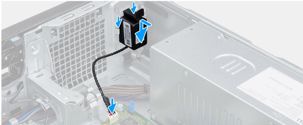
**Figura32. Instalar a coluna**
