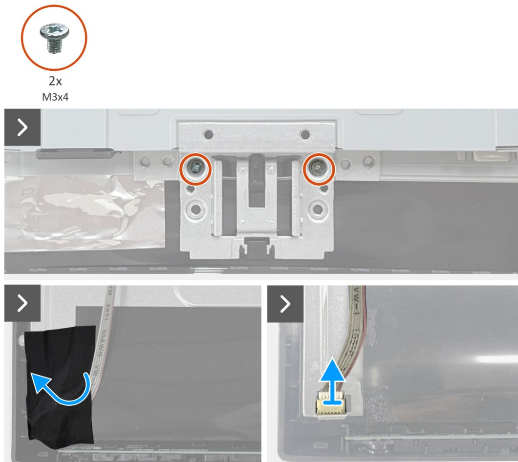
Figura 16. Remover o chassis
