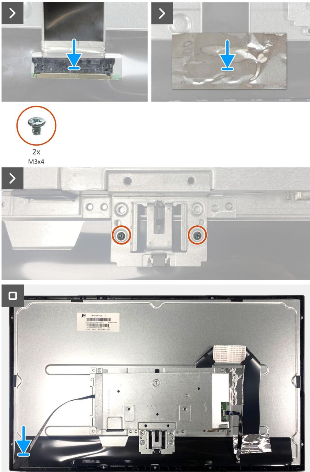
Figura 19. Instalar o chassis
