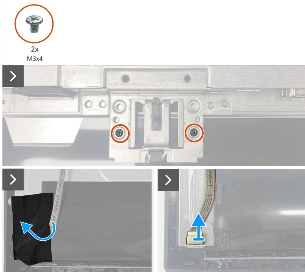
Figura 17. Remover o chassis
