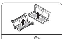
2. Open the outer filter and remove the inner filter (A).
