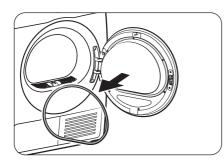
1. Remove the door packing from the door.
