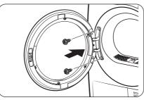
**10.** Insert the door hinge in the opposite position of the door frame, and then, tighten the 2 bolt screws.
