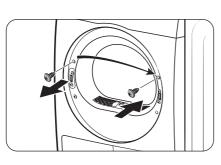
5. Remove the upper screw on the left of the door frame, and then insert it in the corresponding right hole of the door frame. Do not remove the lower bracket screws.
