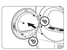
**12.** Tighten the 3 holder screws on the top. Then, tighten the 3 holder screws on the bottom.
