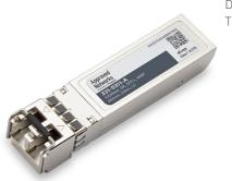
Dell 331-5311 Compatible 10GBase-SR SFP+ Transceiver (MMF, 850nm, 300m, LC Duplex, DDM, I-Temp)
