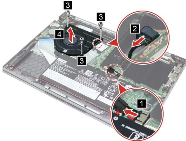
Figure 14. Remove three screws and the fan
