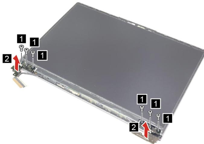
Figure 41. Remove six screws and remove the hinges
