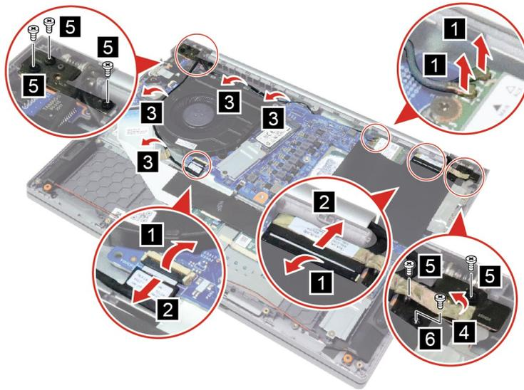
Figure 37. Disconnect cables and remove six screws
