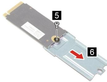
Figure 11. Remove the 2242 solid-state drive bracket
