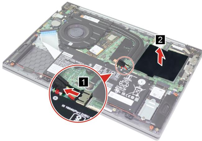
Figure 18. Peel off the memory module mylar
