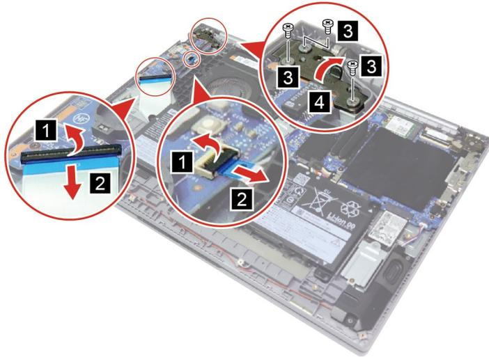
Figure 26. Disconnect the cable(s) and open the hinge
