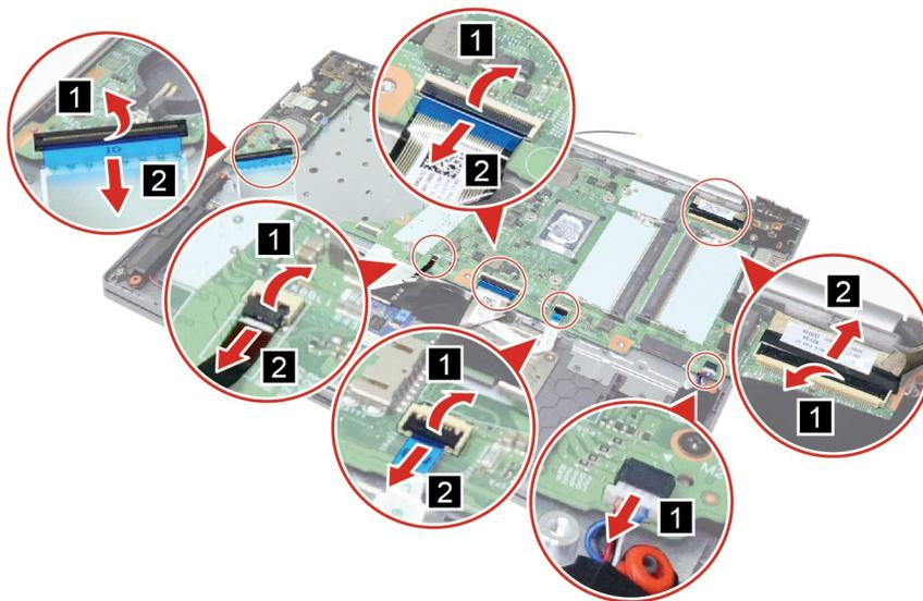
Figure 32. Disconnect cables
