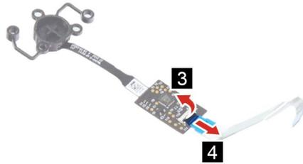
Figure 30. Disconnect the fingerprint reader cable
