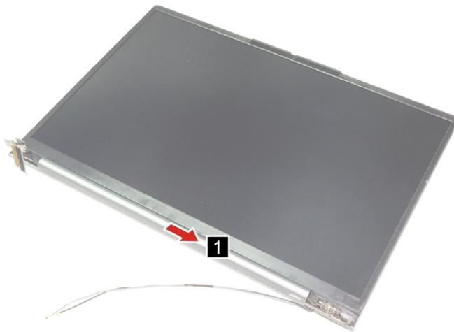
Figure 39. Remove the hinge cover
