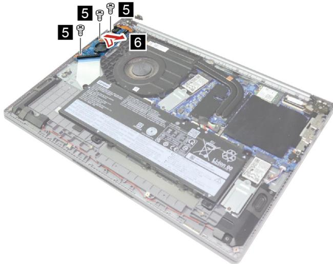
Figure 27. Remove three screws and the I/O board
