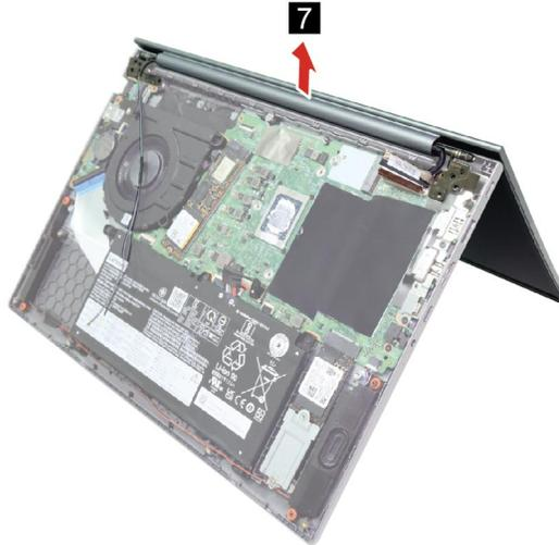
Figure 36. Rotate and remove LCD module
