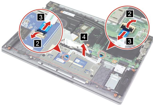
Figure 22. Disconnect and remove the touchpad board cable.
