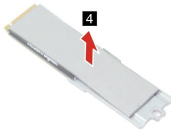
Figure 10. Remove the 2242 solid-state drive thermal pad
