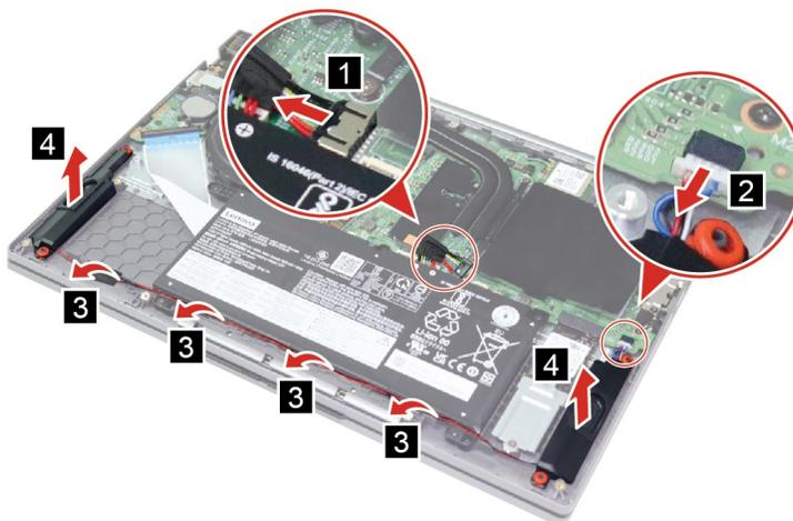
Figure 20. Disconnect cables and remove the speaker
