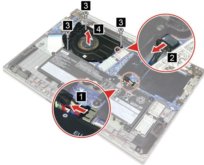
Figure 15. Remove three screws and the fan
