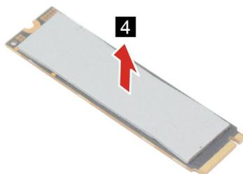
Figure 13. Remove the 2280 solid-state drive thermal pad
