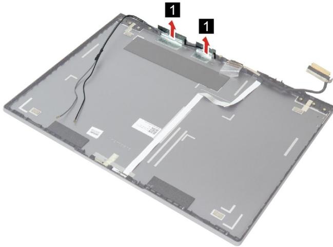
*Figure 50. Remove the antennas*
