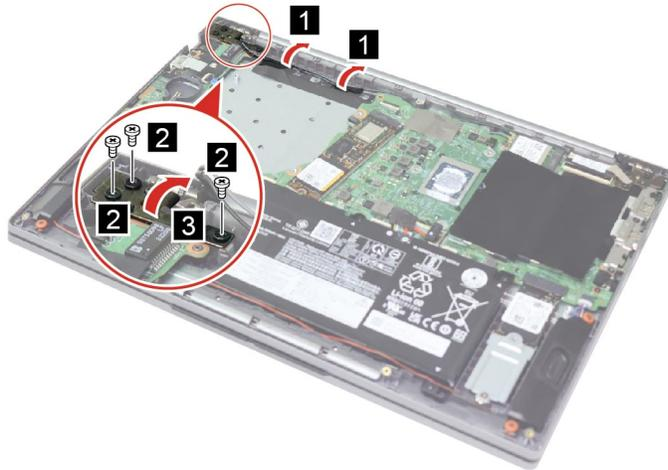
Figure 23. Remove three screws and open the hinge
