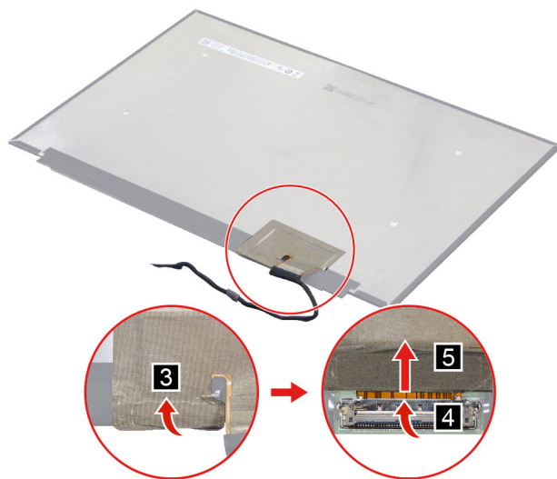
Figure 35. Remove the EDP cable
