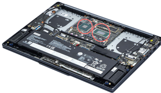
Figure 5. Areas on the system board where thermal interface materials are applied
