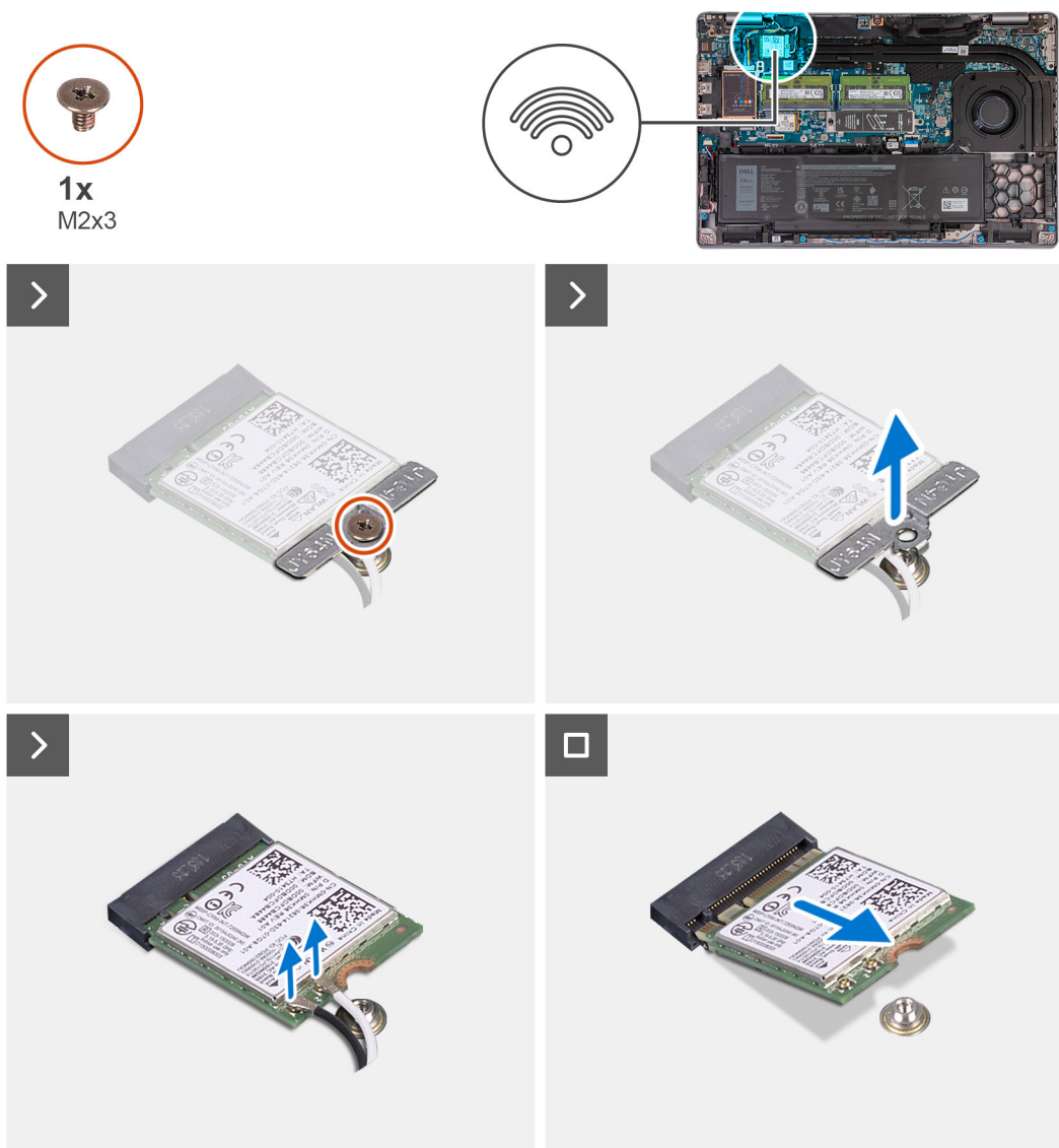
Figure 19. Removing the wireless card
