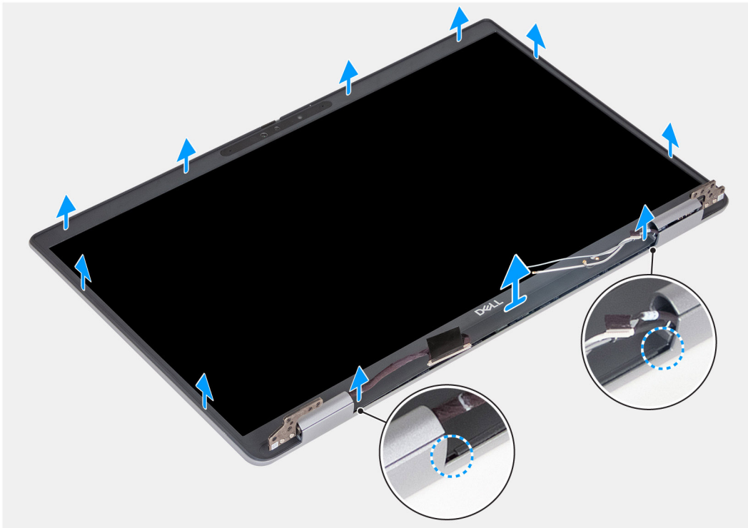
Figure 74. Removing the display bezel
