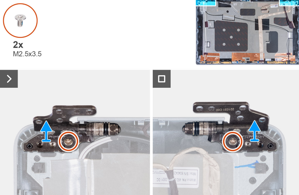
Figure 86. Removing the display hinges
