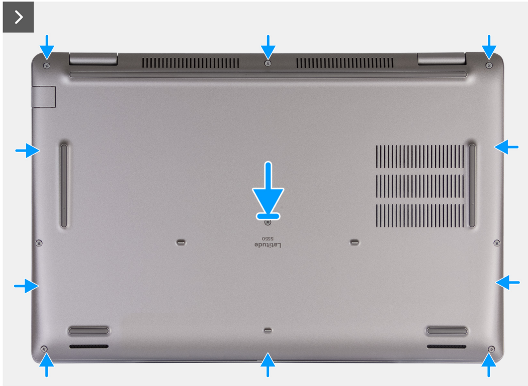
Figure 17. Installing the base cover
