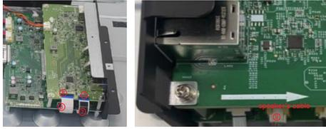
Disconnect IR cable and LED cable from PCBA.
