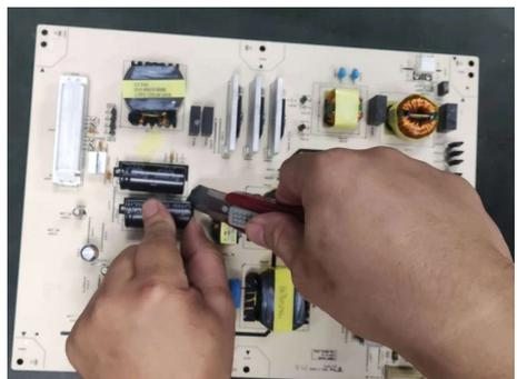
S25-4 Take out bulk cap. pin solder with soldering iron and absorber.
