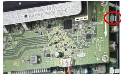
Remove joystick board from the back cover.
