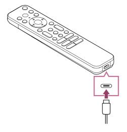
2 Connect the USB Type-C cable to your USB AC adapter.
