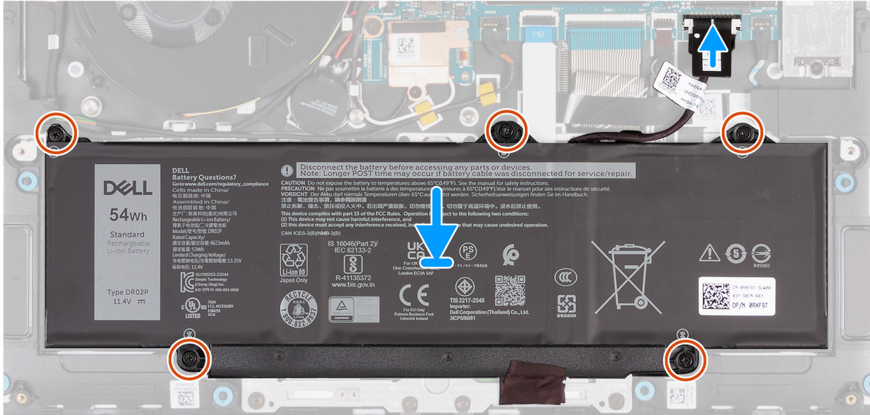
Figure 28. Installing the battery
