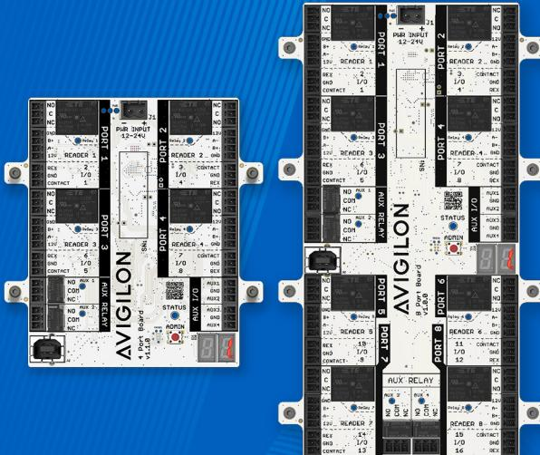
The Avigilon 4-Port and 8-Port Expansion Boards connect to the Avigilon Access Control Core and support either four or eight entries and readers. The Expansion Boards work with the Access Control Core to securely make all entry decisions and include primary ports for Avigilon Smart Readers, relays, request-to-exit (REX) sensors, and contact sensors.
