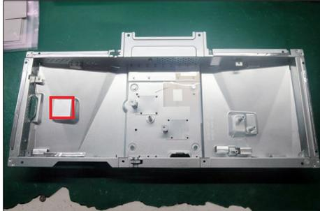
Assemble AC outlet power board to the main chassis.
