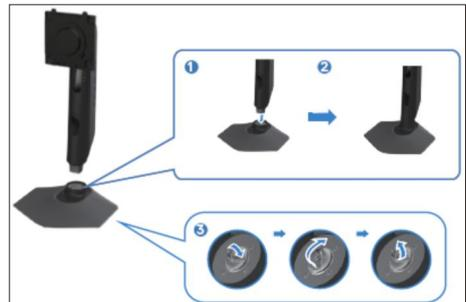
Assemble the stand base with the display monitor.
