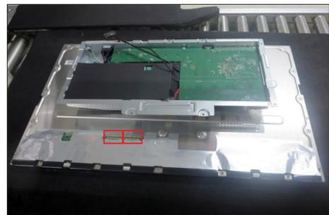
Assemble main chassis to display panel.
