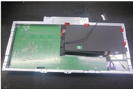
Remove PCBA (interface board and power board).
