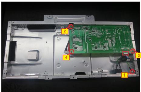
Assemble interface board to the chassis.
