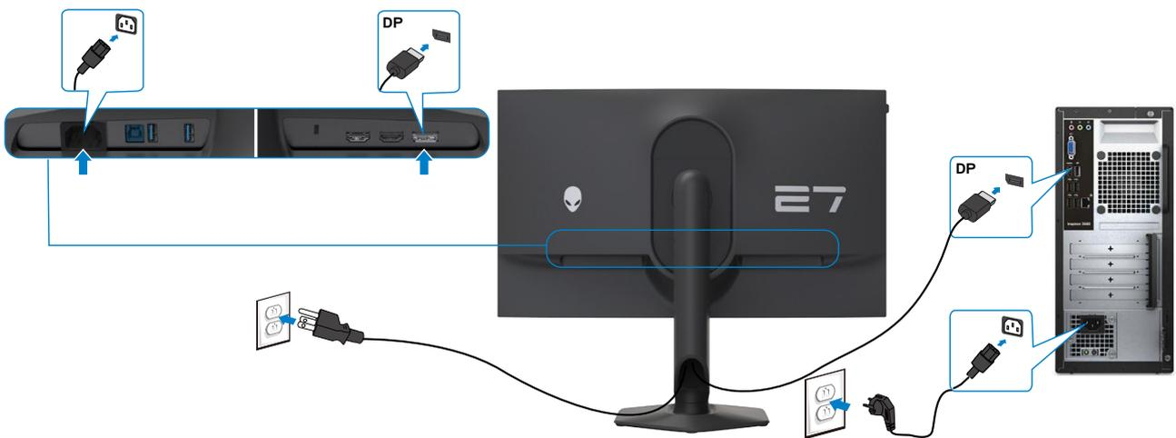
**Figure 4.** Connecting the DisplayPort cable
