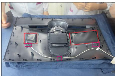
Connect light bar cable to PCBA.
