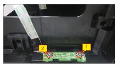
Remove chassis screw and Disconnect eDP cables. a. Remove 4 screws (M3x4) that secure the main chassis.
