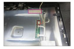
Remove the light bar PCBA.
