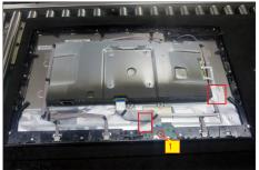
Remove the joystick board. a. Remove 1 screw (M3x6).
