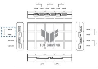
**NOTE:** Fan readings and settings for all fans connected are based off the fan connected to PWM of fan set 1.
