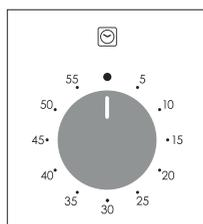
To set the cooking time, turn dial one complete revolution and then position the index to the required time. When the time has lapsed, the signal will ring for a few seconds.
