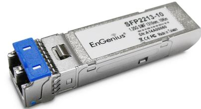
EnGenius Small Form-Factor Pluggable (SFP) transceiver is an industry standard hot-swappable device that plugs into the SFP port or slot and links the port with the network. It is small form factor pluggable module with standard LC duplex connector for fiber communications. It designed to compliant to SFI electrical specifications.
