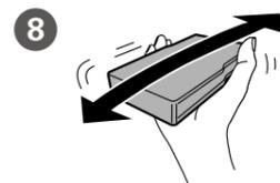
Shake the ink cartridge horizontally for 5 seconds, moving it back and forth about 10 cm 15 times.
