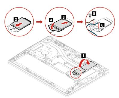
**Note:** When you install the wireless WAN card, ensure that you connect the blue cable to connector **AUX** and the orange cable to connector **MAIN**.
