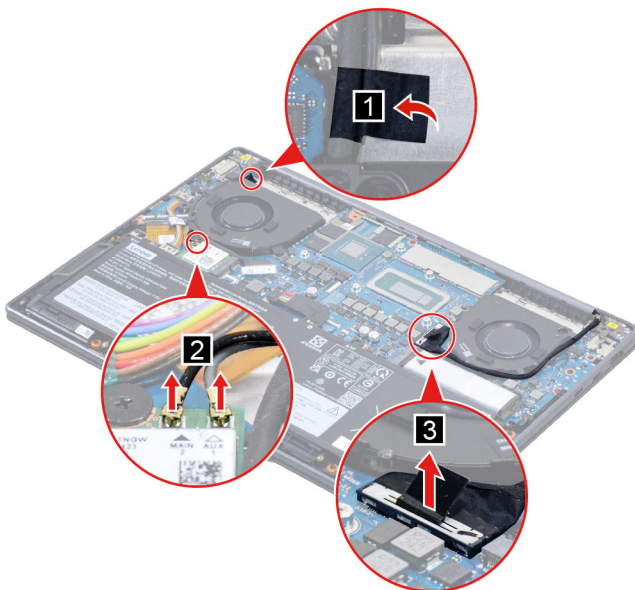
Figure 31. Disconnect the EDP cable and antenna cable
