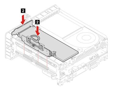
3. Install the screw to secure the PCI-Express card on the computer and install the PCI-Express bracket.
