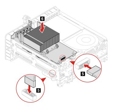
4. Install the MOS heat sink to the PCI-Express card, and secure the PCI-Express card with screws.
