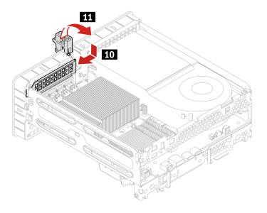
6. Connect the PCI-Express card fan cable and install the fan.
