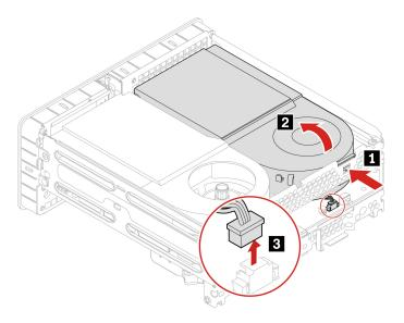
2. Restore the system fan and remove the PCI-Express card fan.
