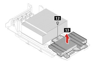
6. Remove the thermal heat sink from the PCI-Express card.
