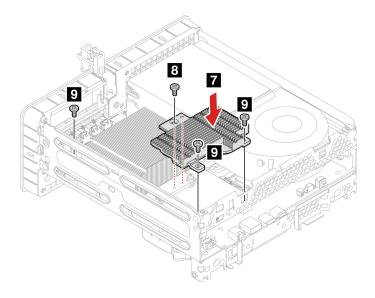
5. Install the PCI-Express card bracket and restore the PCI-Express card latch.
