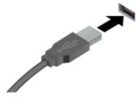
Connect USB-A compatible devices, such as a USB-A keyboard, USB-A mouse, USB-A storage device, or USB-A printer.
