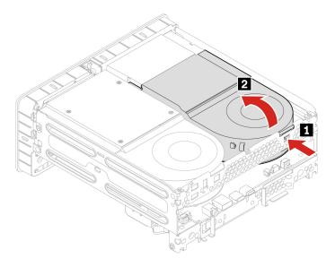
2. Loosen the heat sink screws and remove the heat sink with system fan.
