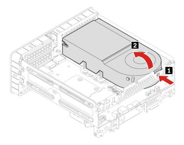
2. Loosen the heat sink screws and remove the heat sink with system fan.
