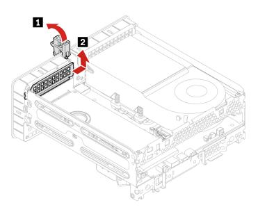
2. Remove one screw and remove the PCI-Express card.
