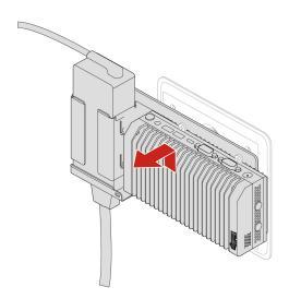
Remove the power cord from the power adapter. See "Power adapter and power cord" on page 59.
