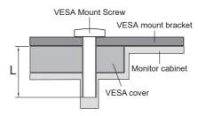
Attach the display arm or desk arm stand to the VESA cover and secure it using the provided VESA Mount Screws or screws of appropriate length.
