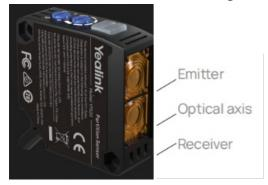
After deployment, the sensor must maintain a distance less than 1.5 meters from the partition. Additionally, when the partition is opened, there should be no structural beams or obstacles behind it that could block the optical path and interfere with its detection accuracy. (Check the details on the Table 1)
