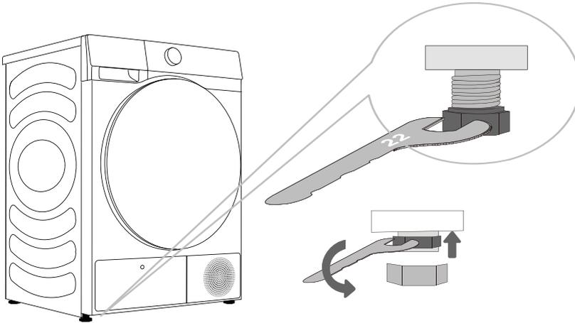
⚠ Floor on which the dryer is placed must have a concrete base. It should be clean and dry; otherwise, the dryer may slide. Also clean the adjustable feet.
