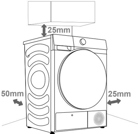
⚠ The dryer may not be in contact with a wall or adjacent furniture. For optimum dryer operation, we recommend observing the clearance from the walls as indicated in the figure. In case of failure to heed the required minimum clearance, the dryer may overheat.
