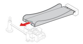
c. Remove the M.2 solid-state drive.
