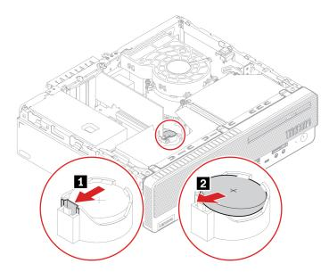
3. Install the coin-cell battery.
