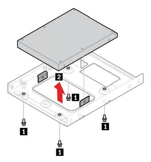
3. Install the 2.5-inch primary storage drive to the storage converter.
