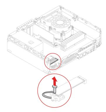
b. Remove the M.2 solid-state drive.
