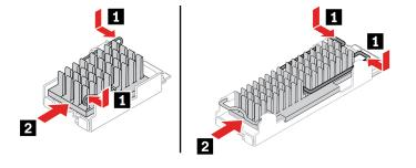
d. Remove the M.2 solid-state drive.
