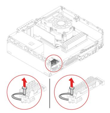
b. Pull out the heat sink with the bracket.
