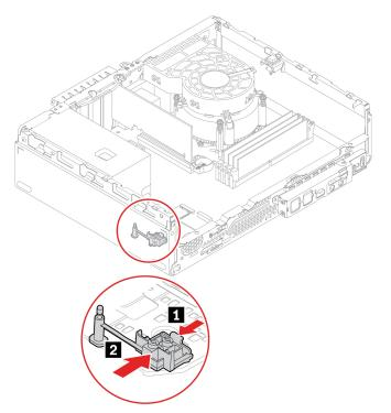
6. Install the M.2 solid-state drive bracket.
