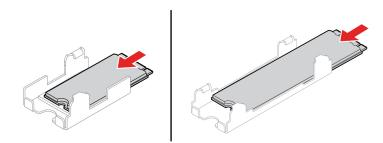
f. Remove the film that covers the thermal pad, if any. Then, install the heat sink.
