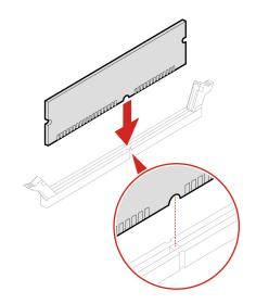
**Note:** During the installation, ensure that you align the memory module to the slot and press down on both ends until the latches are fully engaged with a click.
