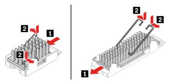
g. Insert the heat sink with the bracket.
