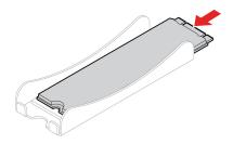
e. Insert the heat sink with the M.2 solid-state drive.
