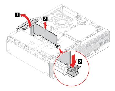
3. Remove the PCI-Express connector cable, if any. See "PCI-Express connector cable" on page 52. Then, install the PCI-Express card.
