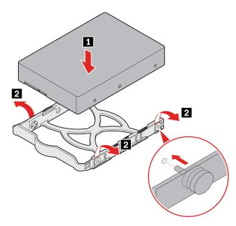
8. Install the 3.5-inch primary storage drive with the bracket.
