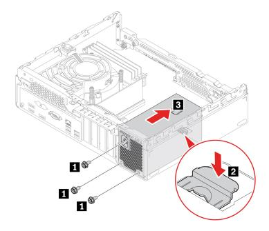
6. Install the power supply assembly.
