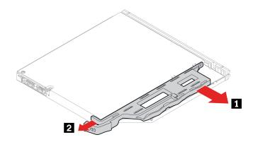
6. Install the optical drive bracket.
