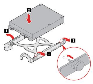
9. Install the 2.5-inch secondary storage drive with the bracket.
