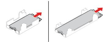
e. Remove the film that covers the thermal pad, if any. Then, install the M.2 solid-state drive.
