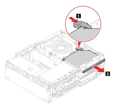
5. Remove the optical drive bracket.
