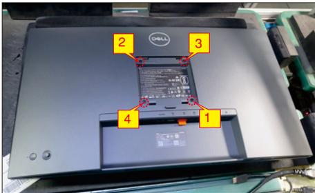
Wedge your fingers between the rear cover and the middle bezel on the corners of the top side of the monitor to release the rear cover, then use one hand to press the middle bezel, the other hand to pull up carefully the rear cover in order of arrow preference for unlocking mechanisms of rear cover.
