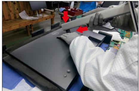
Lift up the monitor, then provide power supply and a video signal to the monitor, then turn on the monitor for functionality check.
