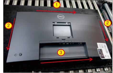
**S6** Lift the rear cover up carefully. Disconnect the joystick cable from the connector of the interface board, and then remove the rear cover.
