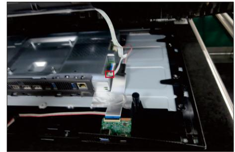
**S7** Put the rear cover into a fixture jig, then release the key cable by tearing off the tapes. Use a Philips-head screwdriver to remove 1pcs screws for unlocking the joystick key board with the rear cover.
