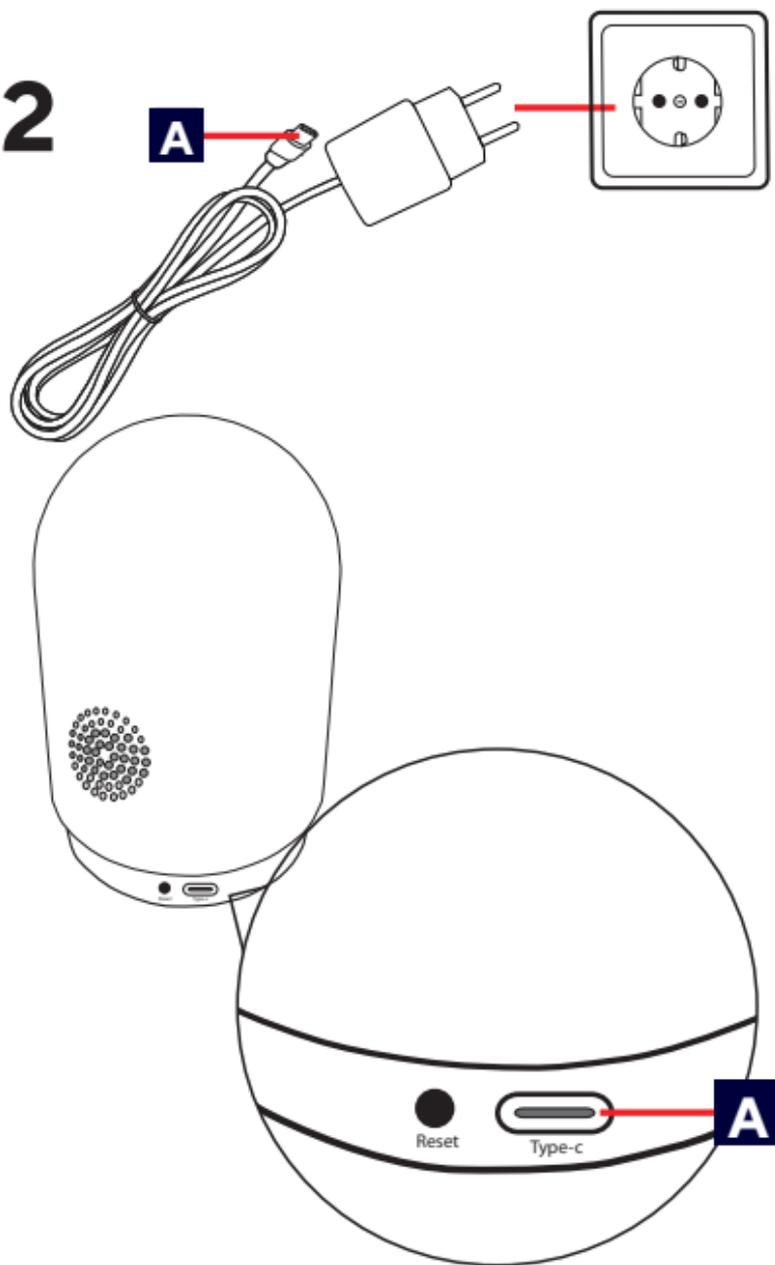
**A** Connect the supplied USB-C power cable to the back of the camera
