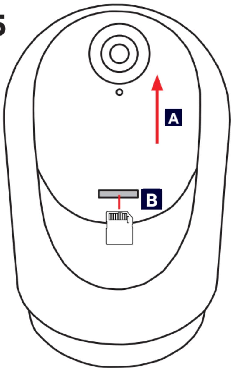
**A** Manually move the camera lens up or use the PTZ control in the App.
