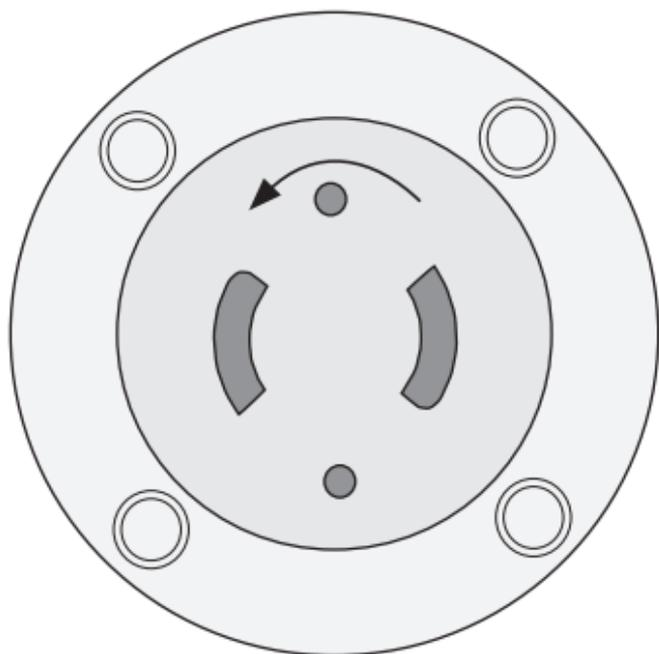
Remove mounting plate by rotating it counterclockwise from the bottom of the camera
