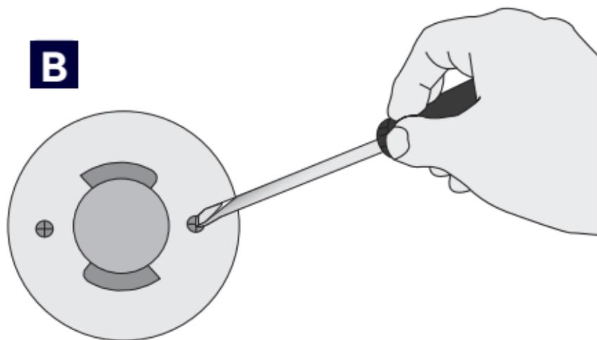
Secure the mounting plate on a flat surface using the supplied wall plugs and screws.
