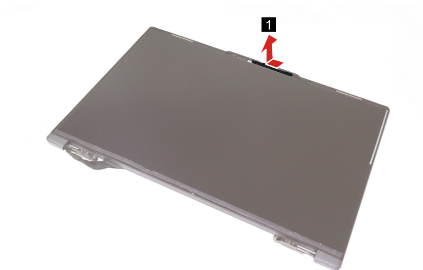
Figure 41. Remove the camera shutter
