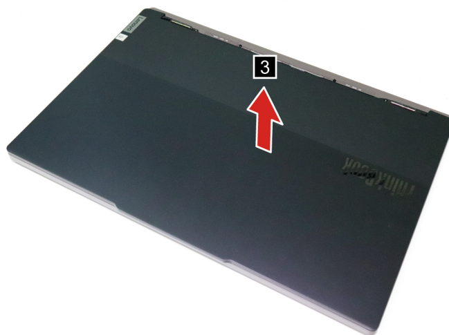
Figure 38. Remove the LCD unit
