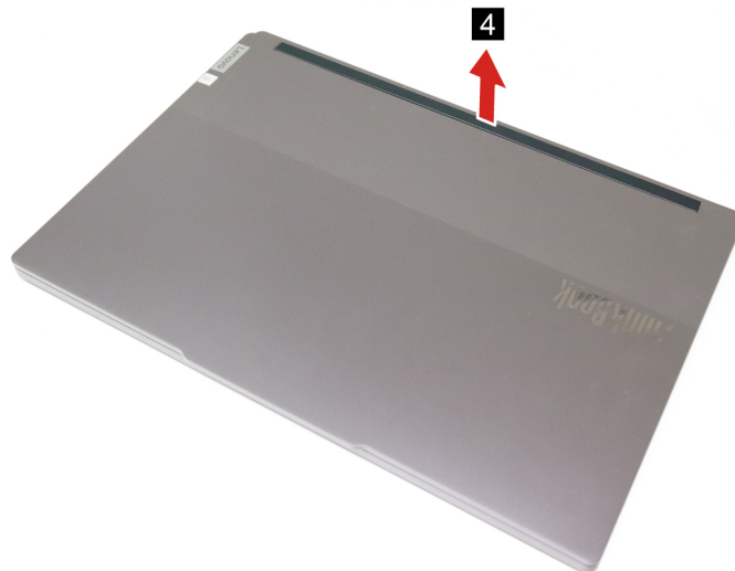
Figure 29. Remove the hinge cap
