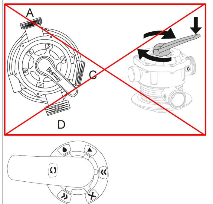
Press down on the control valve handle and rotate to desired function. To prevent equipment damage , always switch the sand filter off before changing the control valve function.
