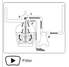
This function is used to filter pool water and should be positioned here 99% of the time. Water is pumped through the sand filter, where it is cleaned and returned to the pool.
