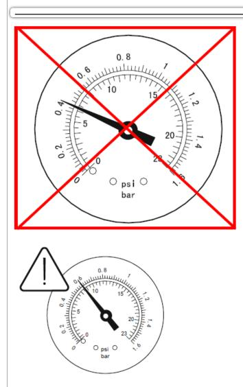
**CAUTION:** You must ensure the sand filter is switched off and unplugged before starting any maintenance or there is a severe risk of injury or death. As dirt builds up in the sand filter, the pressure reading on the Pressure Gauge will increase. When the Pressure Gauge is 0.45 Bar (6.5 PSI) or higher, it is time to clean the sand. To clean the sand bed, follow all instructions outlined previously in: **Backwash and Rinse**.
