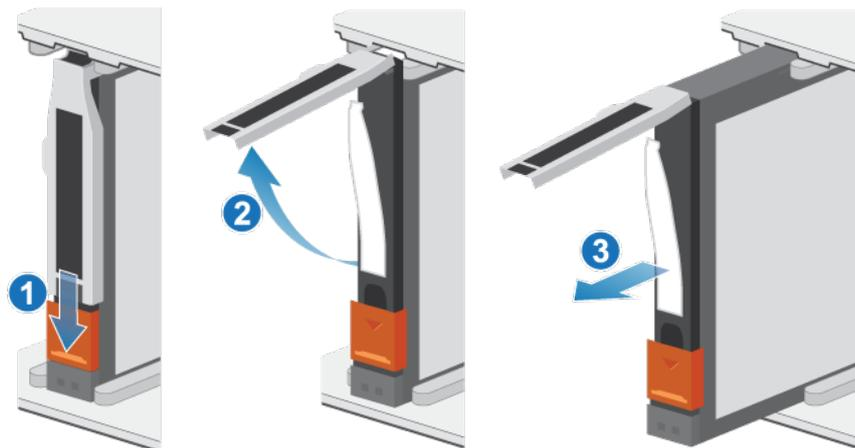
Figure 101. Removing a drive
