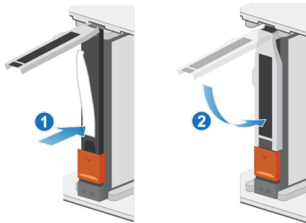
Figure 21. Installing a drive
