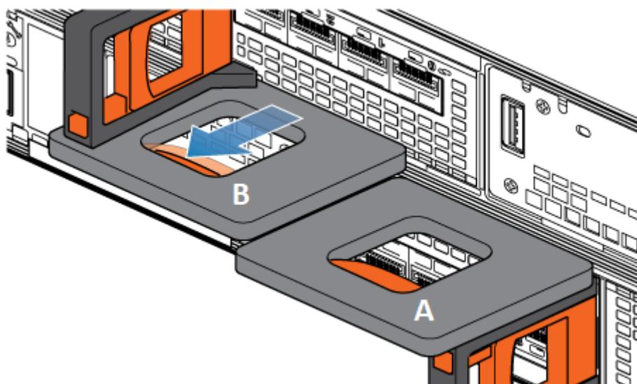
**Figure 90. Disengaging the locking mechanism for node B**
