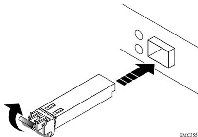
Figure 63. Installing an SFP module
