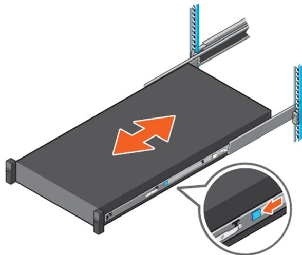
**Figure 29. Slide system into the rack**
