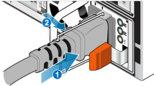
Figure 5. Inserting the power cable
