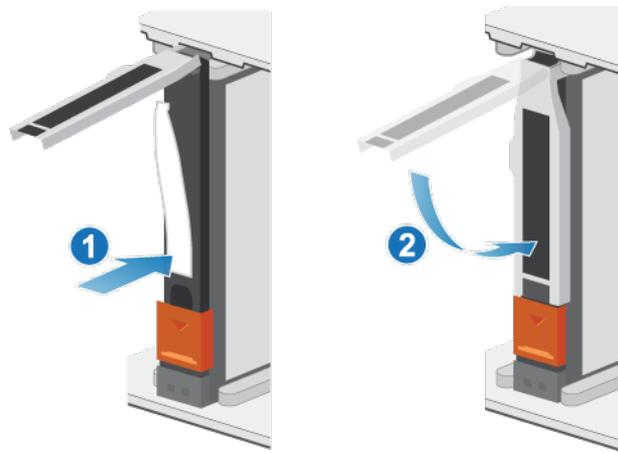
Figure 106. Installing a drive
