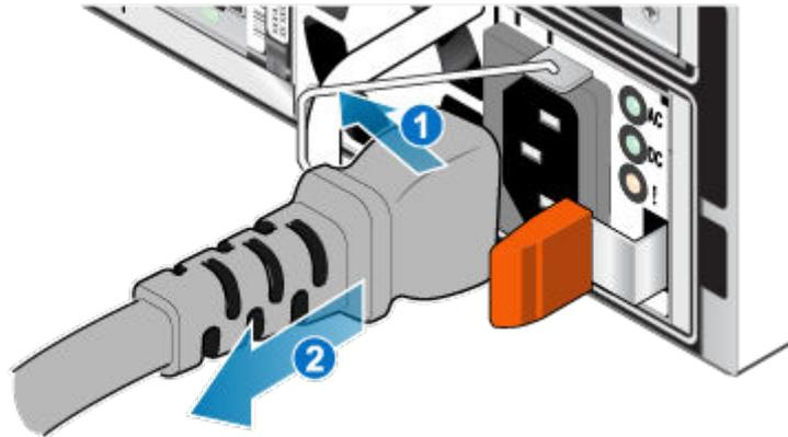
Figure 79. Removing the power cable
