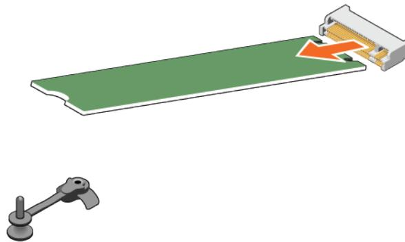
**Figure 94. Removing the internal M.2 boot module**
