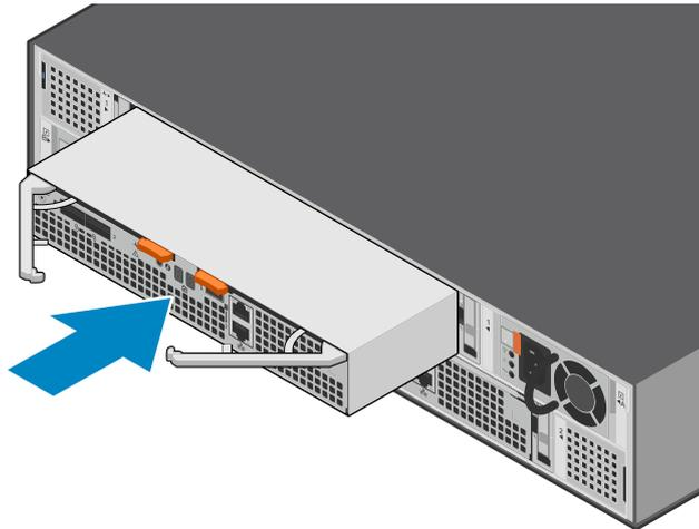
**Figure 123. Installing the Access Module**
