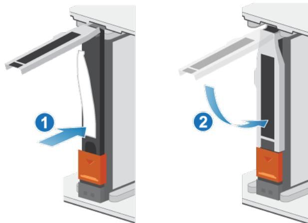
Figure 37. Installing a 2.5" drive
