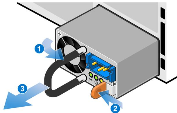
Figure 47. Removing a DC power supply
