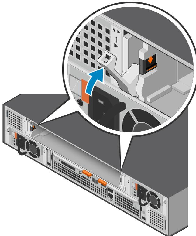
Figure 128. Locking the DIB into place
