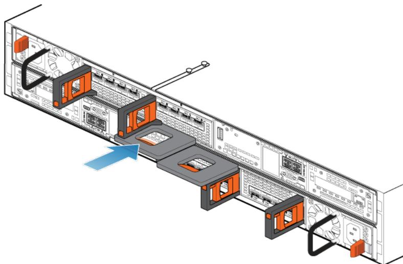
Figure 61. Installing the node
