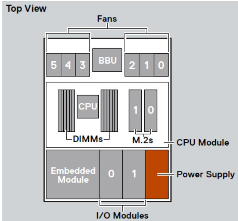
Figure 83. Top view of the node
