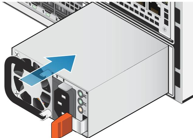
Figure 43. Installing a power supply
