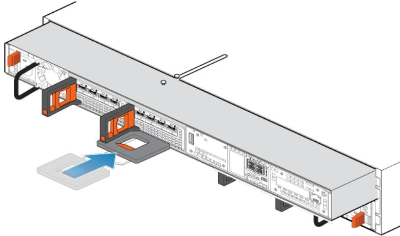
Figure 60. Sliding the node halfway into the chassis
