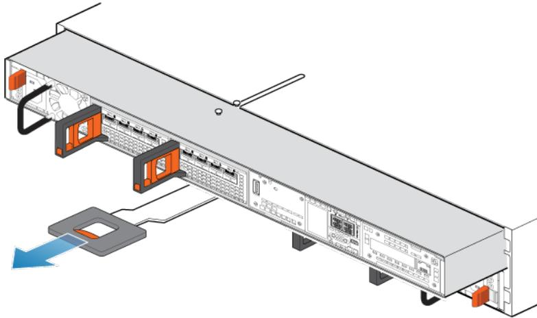
**Figure 81. Removing the node**
