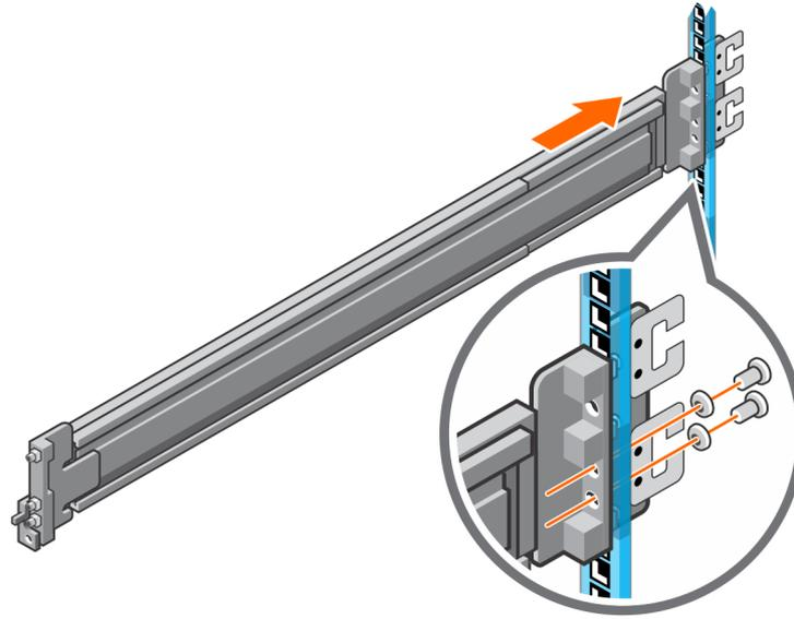
**Figure 23. Installing the NVMe expansion enclosure rails (rear)**
