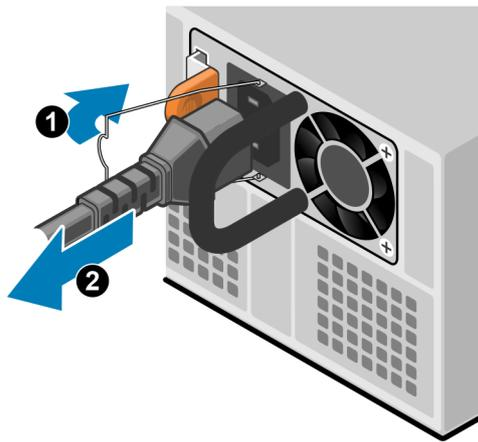
**Figure 109. Removing the power cable**
