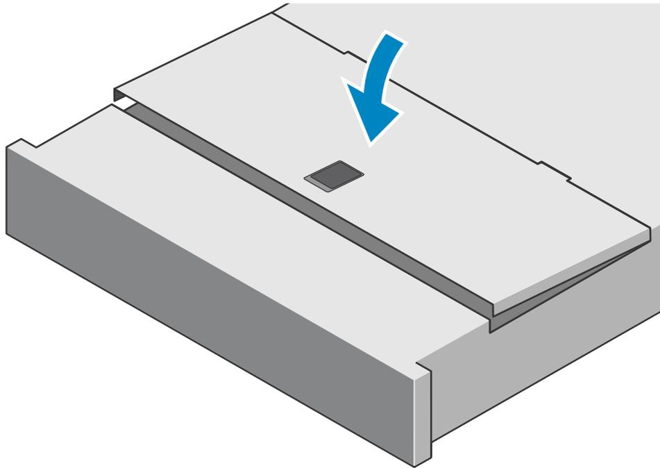
**Figure 116. Closing the system cover**
