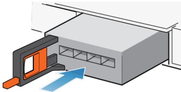
Figure 67. Installing an I/O module
