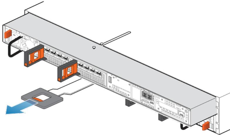
**Figure 91. Removing the node**
