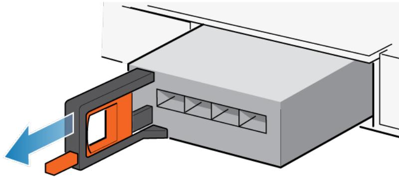
Figure 66. Removing the I/O module
