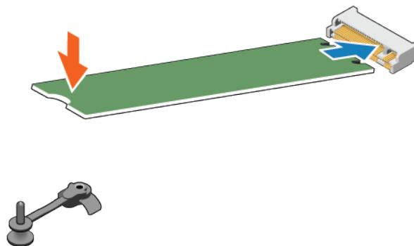
**Figure 95. Placing the internal M.2 boot module**
