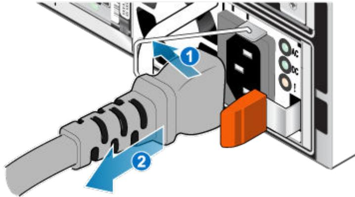
**Figure 51. Removing the power cable**
