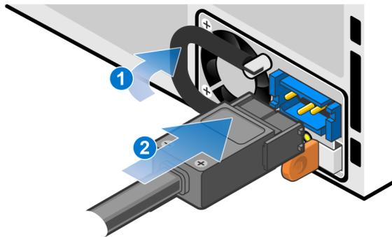
**Figure 49. Inserting a DC power cable**
