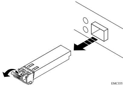
Figure 62. Removing an SFP module
