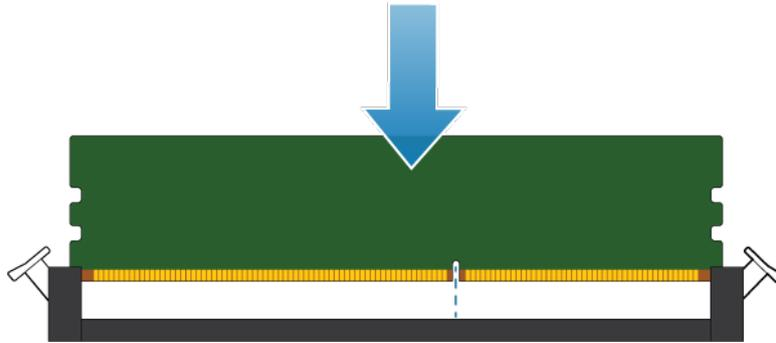
**Figure 85. Installing the DIMM**
