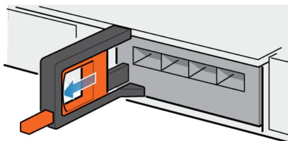
Figure 65. Releasing the I/O module
