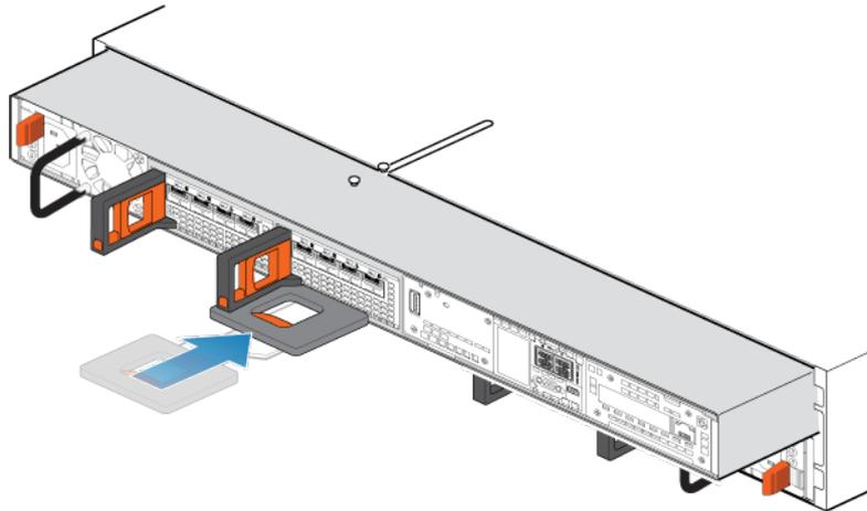
**Figure 77. Sliding the node halfway into the chassis**
