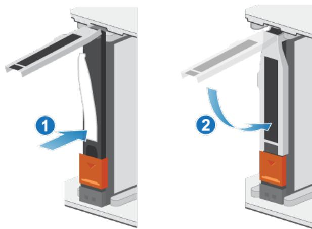
Figure 34. Installing a drive
