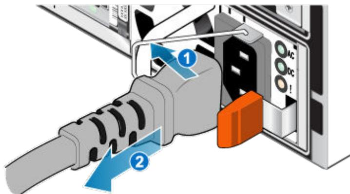
Figure 41. Removing the power cable
