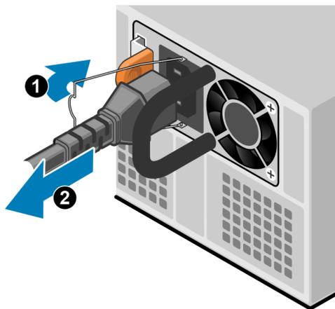
**Figure 110. Removing a power supply**
