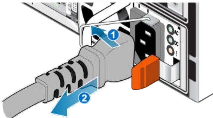
Figure 69. Removing the power cable
