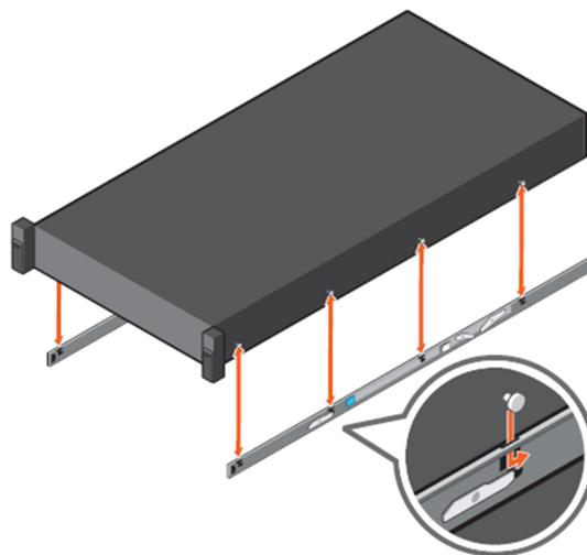
**Figure 27. Attach the inner rails to the system**
