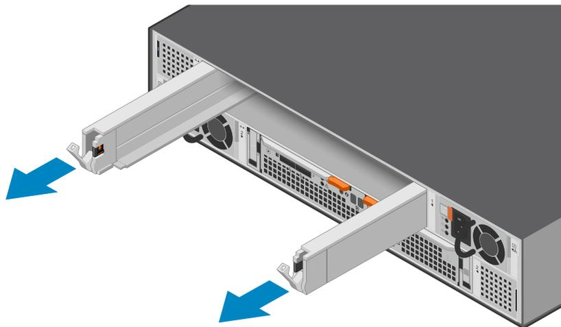
**Figure 126. Removing the DIB**
