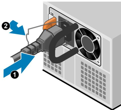
Figure 112. Inserting the power cable
