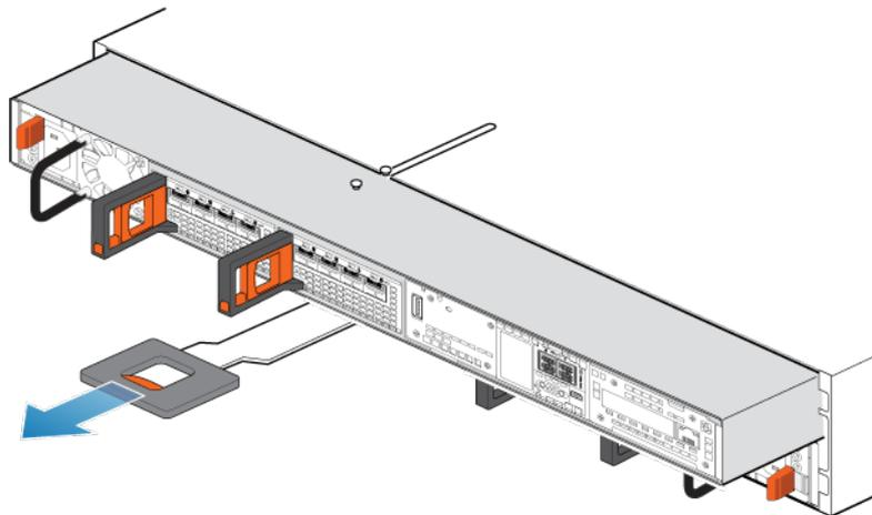
**Figure 71. Removing the node**
