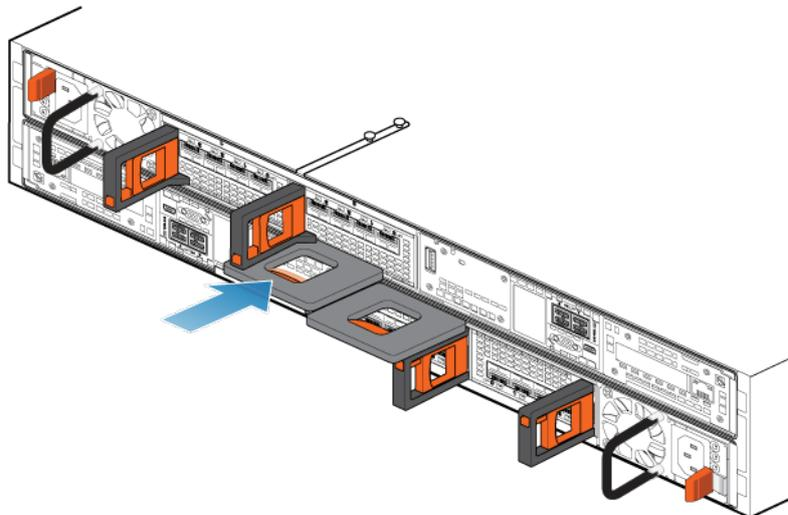
Figure 88. Installing the node
