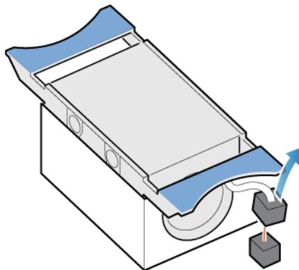
**Figure 73. Disconnecting the fan power cable**
