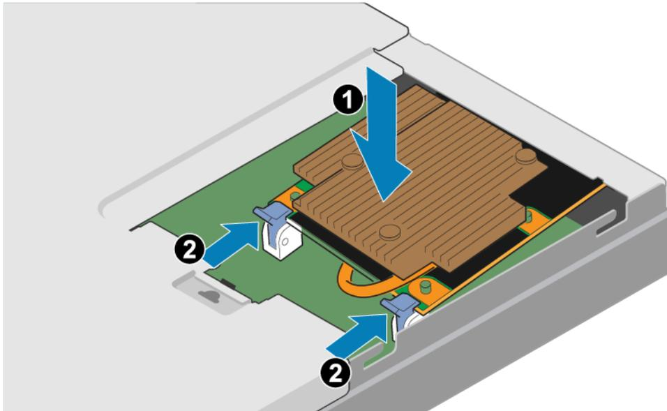
**Figure 58. Locking the 4-port card into position**
