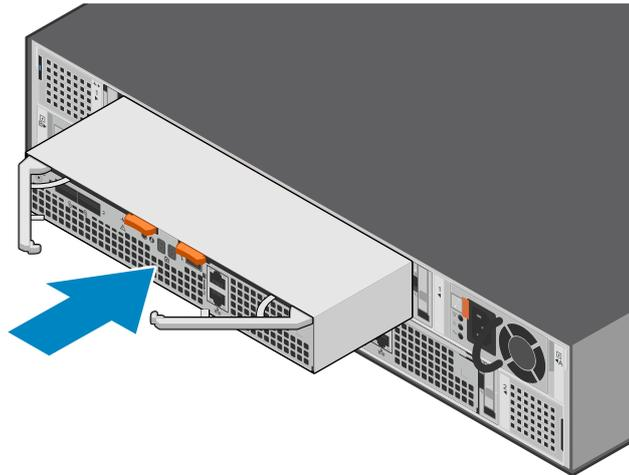
**Figure 134. Installing the Access Module**
