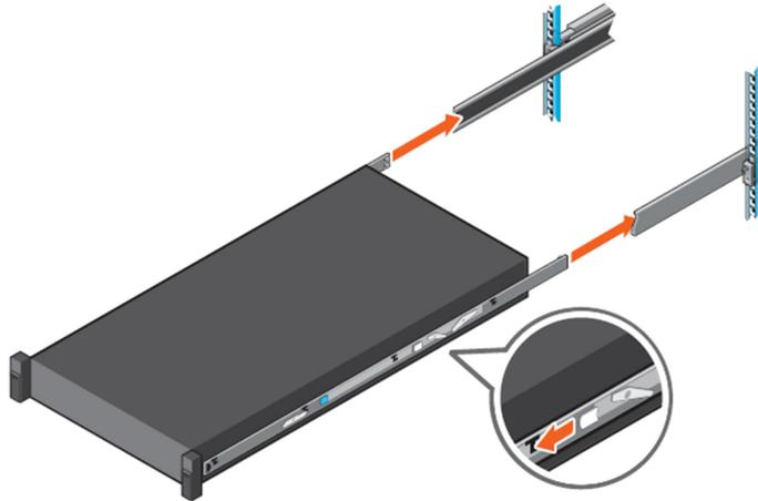
**Figure 14. Install system into the extended rails**
