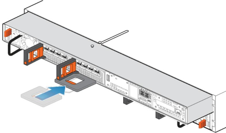
Figure 87. Sliding the node halfway into the chassis
