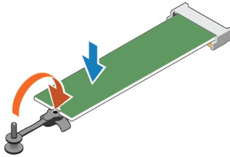
Figure 96. Connecting the internal M.2 boot module to the motherboard
