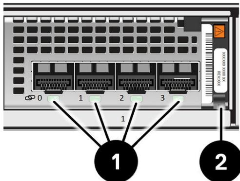
Figure 64. Base enclosure I/O module LEDs
