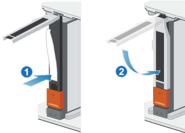
Figure 102. Installing a drive
