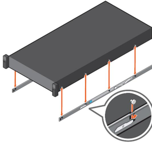
**Figure 13. Attach the inner rails to the system**
