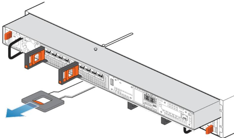
**Figure 53. Removing the node**
