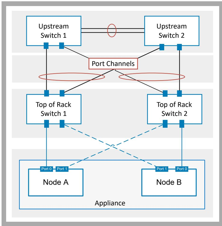
Figure 4. ToR switches with no direct interconnect
