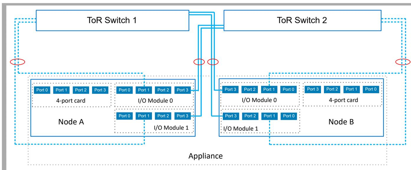
Figure 18. Sample configuration for a Fail Safe Network
