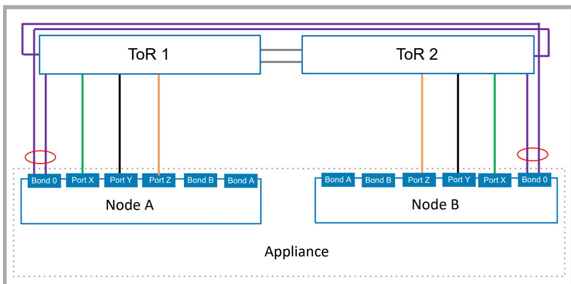
Figure 5. Network connectivity for Block-optimized storage networks
