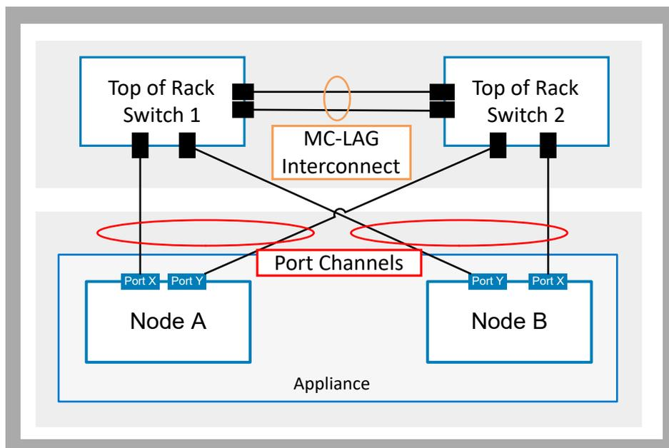
**Figure 1. ToR switches with MC-LAG interconnect**
