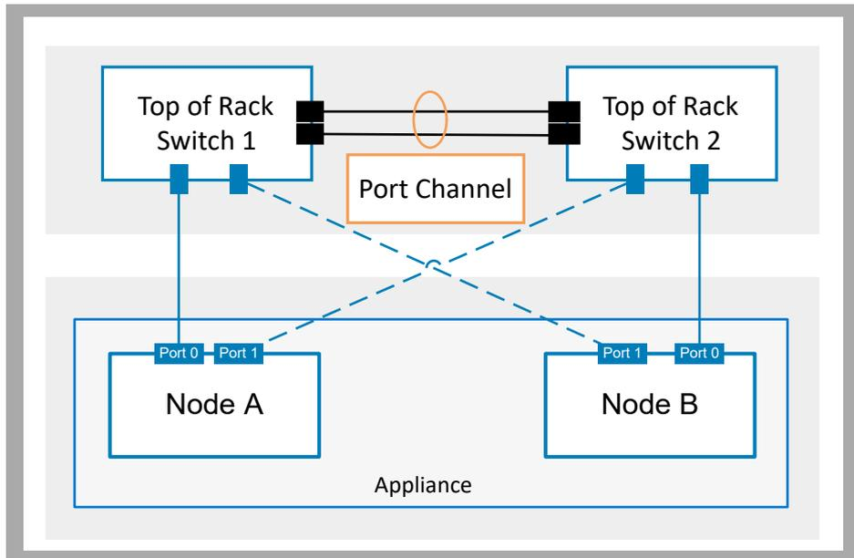
**Figure 3. ToR switches direct interconnect not using MC-LAG**
