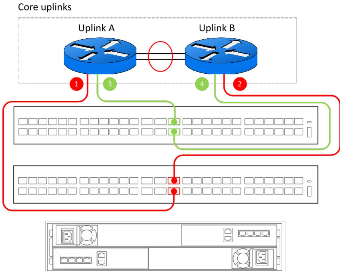
**Figure 11. Dell PowerSwitch Series S4148-ON ToR switch connections to the core uplinks**
