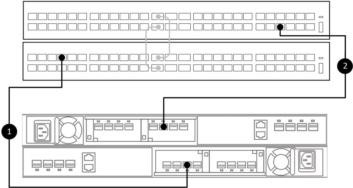
**Figure 12. Connect node ports to the ToR switches for the iSCSI and Replication and Block Import networks**
