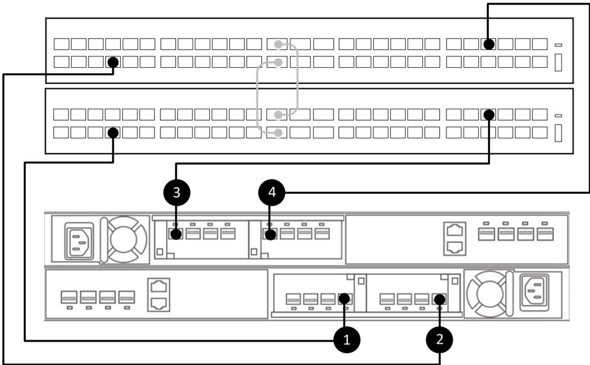
**Figure 14. Connect node ports to the ToR switches for the NAS network**
