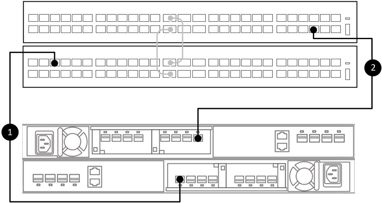
**Figure 13. Connect node ports to the ToR switches for the NVMe/TCP network**
