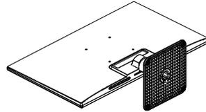
2. Press the release button to detach the base column.
