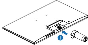
2. Hold the monitor base stand with both hands and firmly insert the base stand into the base column.
