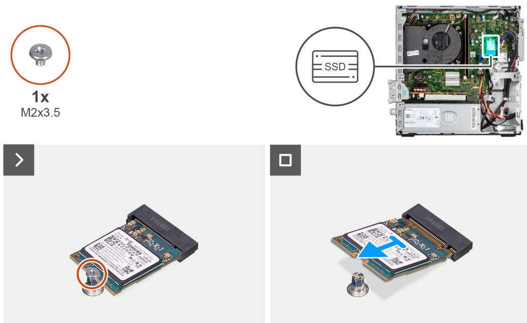
Figure 17. Removing the M.2 2230 solid-state drive
