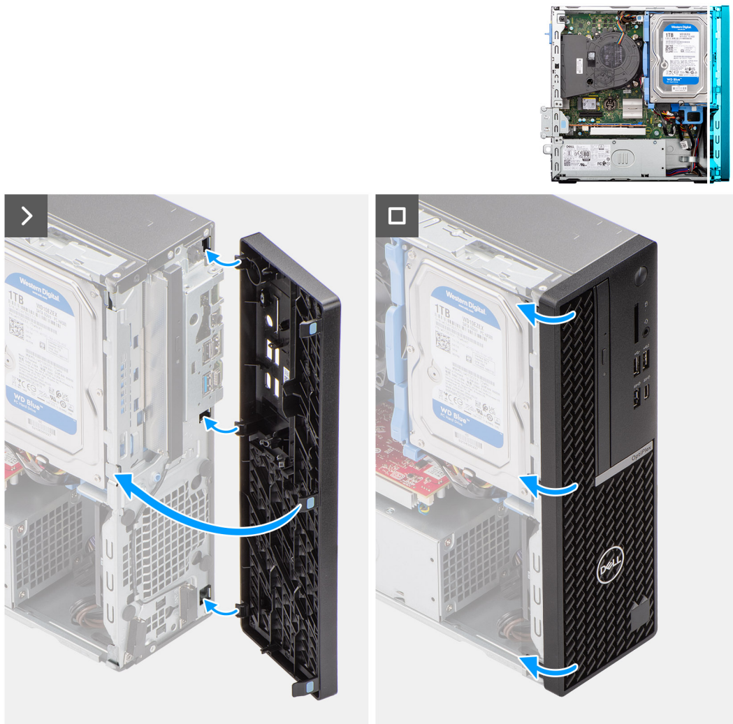
Figure 8. Installing the front bezel
