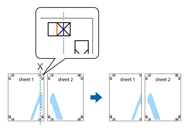
2. Place the edge of Sheet 1 on top of Sheet 2 and align the cross marks, then temporarily tape the two sheets together from the back.
