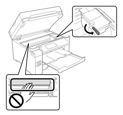
9. Secure the print head to the case with tape.
