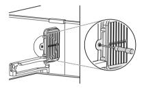
3 Press on the hooks on the deodorizer and remove it.
