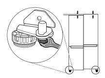
1 Open the door and use the spanner 1 to loosen the keeper nut by turning it to the left.
