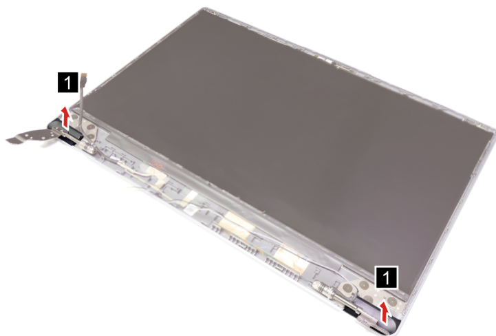
Figure 40. Remove the hinge covers
