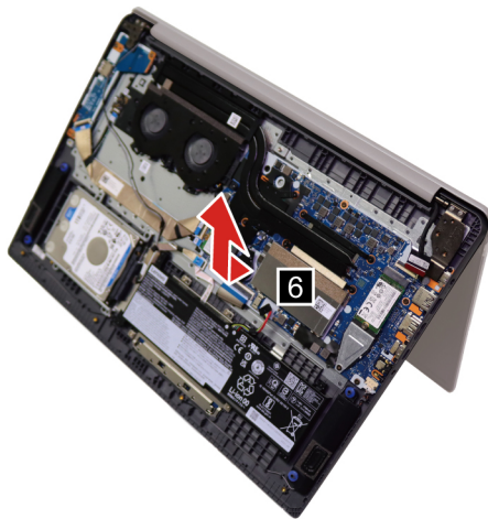
Figure 38. Remove the LCD unit
