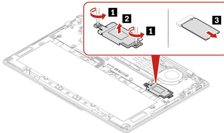
Step 2. Install the M.2 solid-state drive and M.2 solid-state drive bracket in reverse order.
