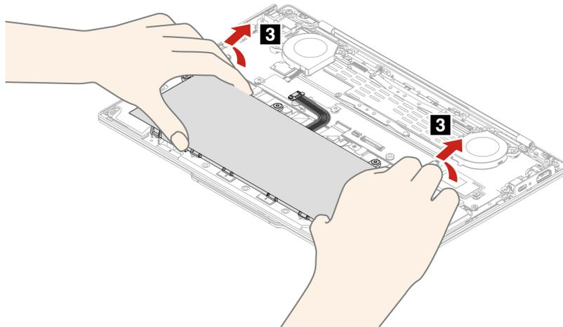
Step 2. Before installing the built-in battery, thoroughly check the battery compartment and ensure that there are no foreign or sharp objects that could cause damage to the battery.
