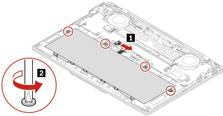
b. Remove the battery as shown below.
