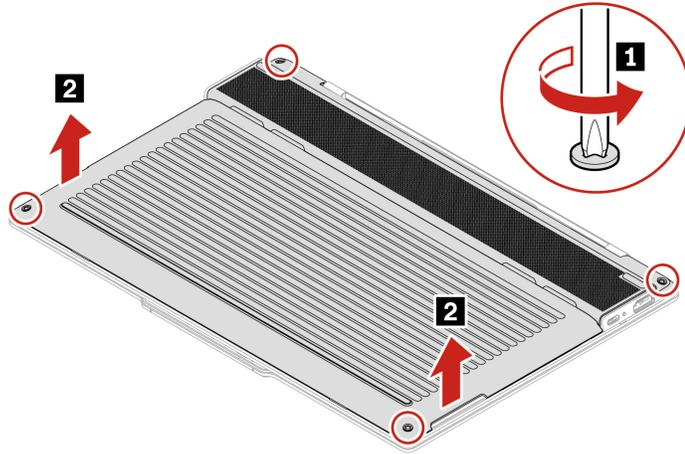
Step 2. Install the assembly as shown below.
