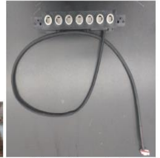
Take out the controller assembly to complete switch dismantling
