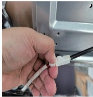
Pull out the spotlight terminal
