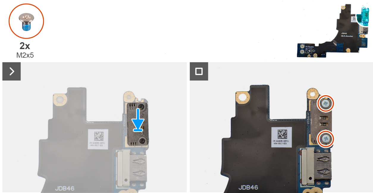
Figure 53. Installing the left USB Type-C module
